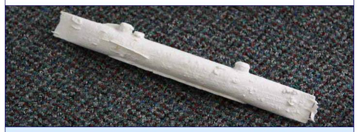
multi-billion point data cloud created with a precision laser scanning the real sub and then printing that data with a 3 dimensional printer. The model is about one foot long and shows to exact detail
