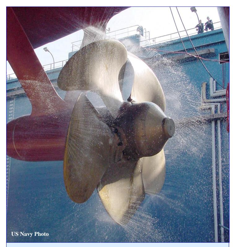
Five bladed screw on an Arleigh Burke class destroyer in drydock testing the water/air system which ejects through the blade tips to quench the noise normally associated with a powerful screw thrusting at the ship's rated power. The system works, making this class destroyer the most silent surface warfare vessel afloat. (Until the USS Zumwalt class [3 ships] joins the fleet.)
